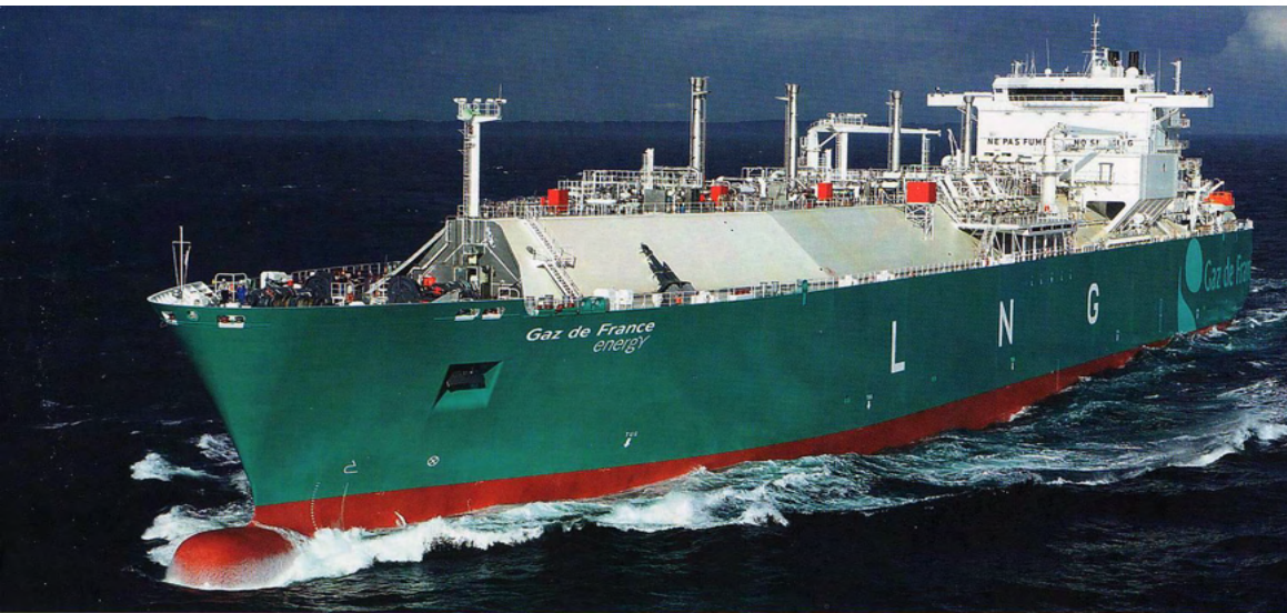
Fig. 5 The LNG carrier, the 75,000m 3 Gaz de France Energy, is equipped with four 6-cylinder Wärtsilä 50DF engines.
